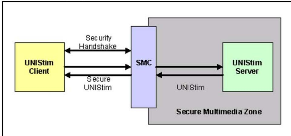
UNISlim security enhances the basic UNISlim protocol by providing Advance Encryption Standard (AES) 128-bit encryption for confidentiality and an AES-based Message Authentication Code for authentication and integrity.
