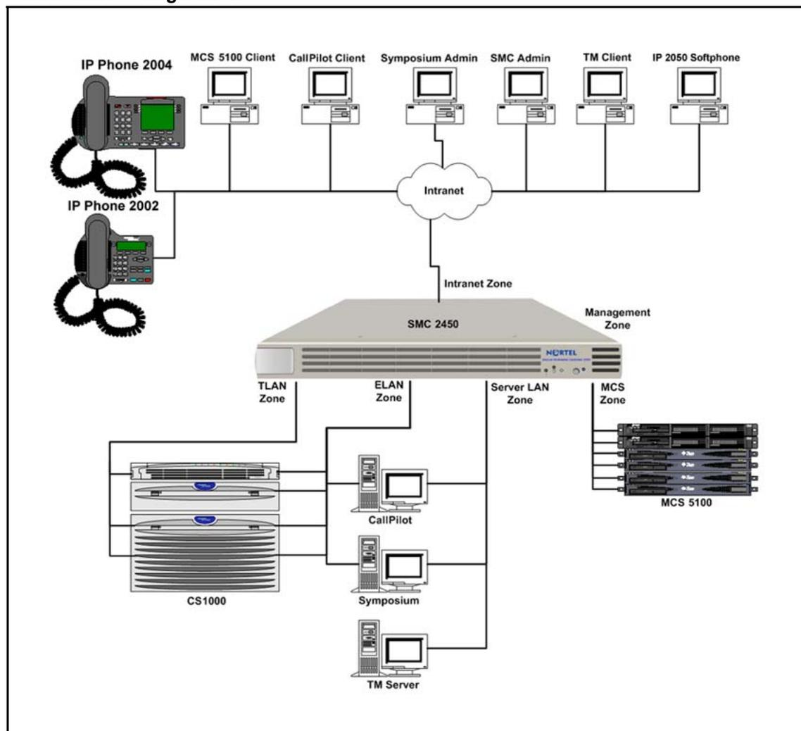
The management network needs two IP addresses in the stand-alone configuration. The first address is the host IP address, which is the IP address for the SMC. The second IP address is the cluster Management IP (MIP) address. Users communicate with the SMC using the cluster MIP address.
