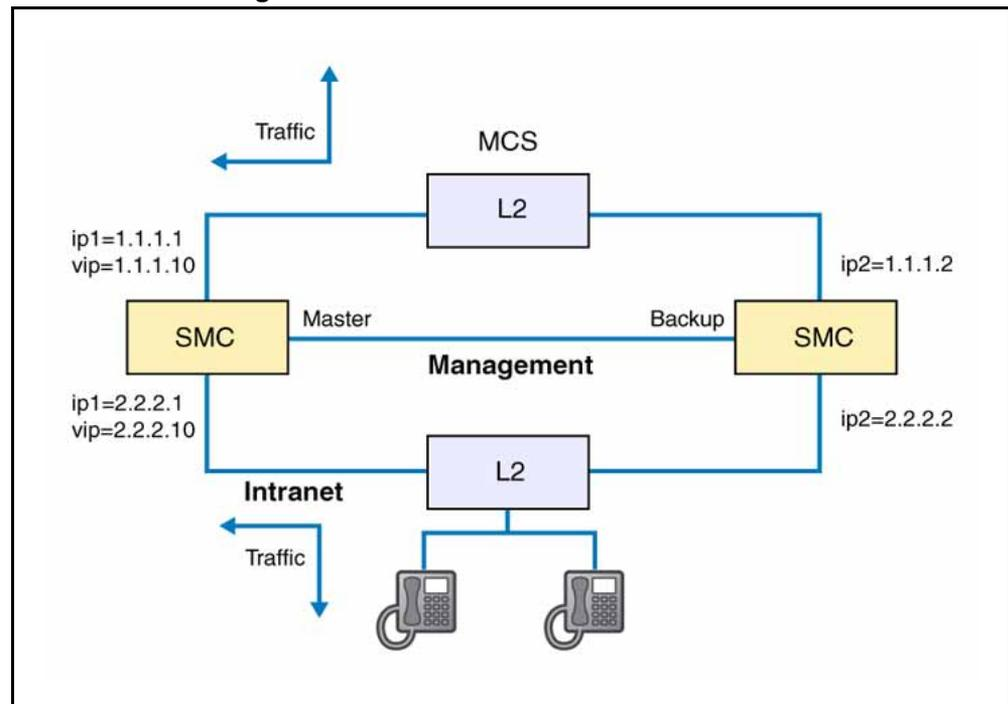
In all routing tables in external devices, use the floating IP address to route packets. The floating IP address is always available even when one SMC in the cluster fails.
