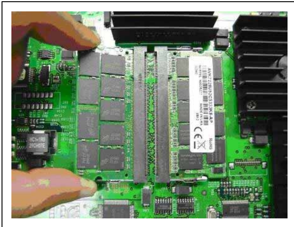
Figure 173 Inserting a memory module in CP PM card
