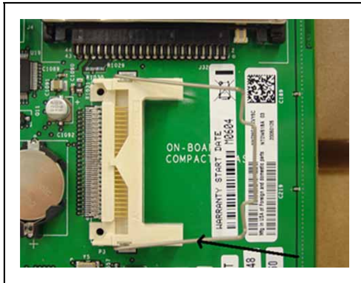
Figure 170 CP PM Signaling Server internal CF card retainer clip
