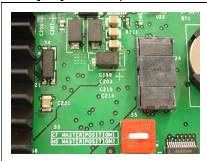
Figure 169 CP PM Signaling Server FMD dip switch
