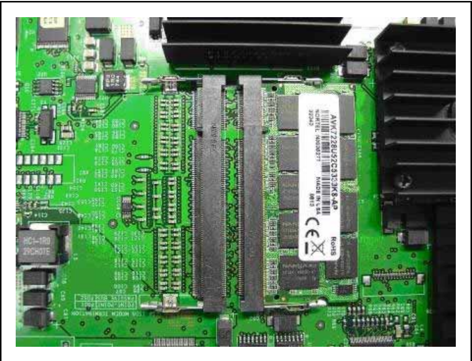
Figure 172 CP PM card with empty memory slot
