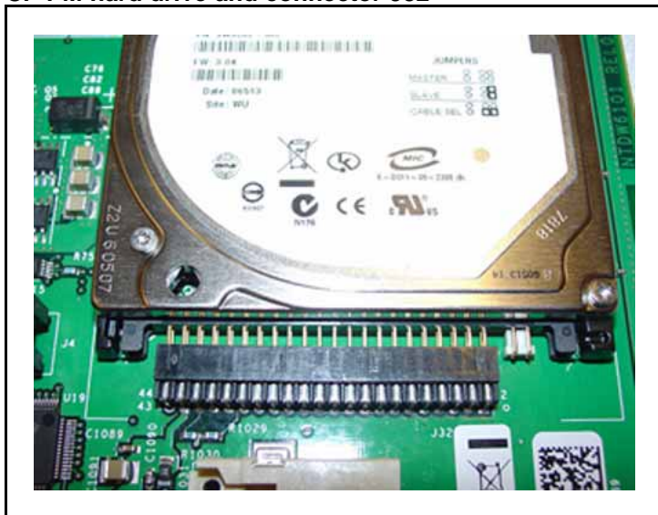
Figure 167 CP PM hard drive and connector J32
