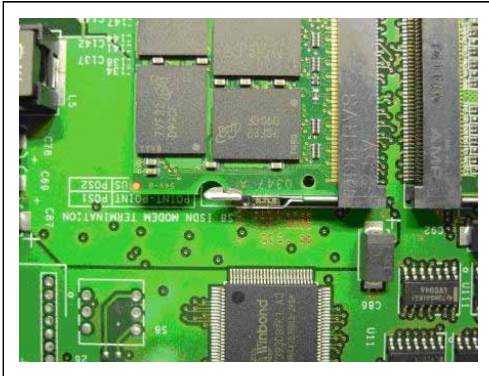
Figure 174 Fastening memory module in CP PM card
