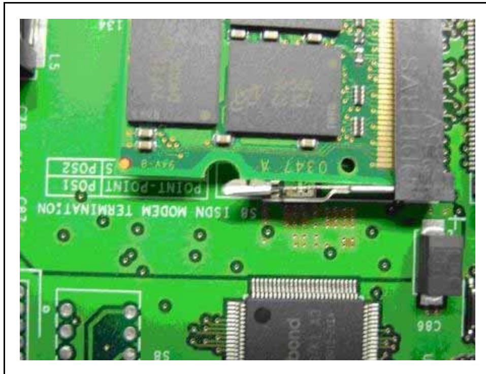
Figure 175 Incorrectly aligned memory module
